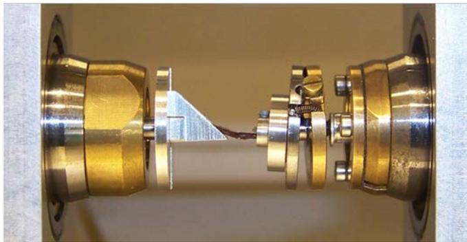
Figure 2. the spider tarsus-metatarsus joint placed in the Tomopress in-situ compression tester. The wedge on the left allows to control the angle between the tarsus and the meta-tarsus without application of additional external load. The magnetic sample holder on the right allows to control the orientation of the leg-joint in the beam path. The chamber was sealed with kapton foil and a humidity generator was used to maintain constant humidity level.
