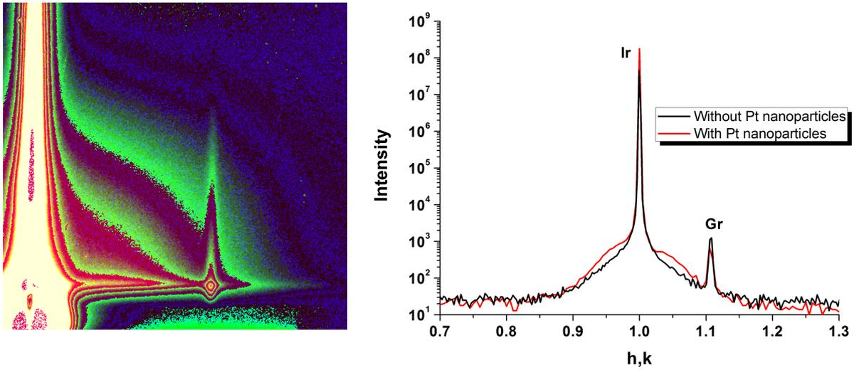
Fig. 1: (Left) GISAXS pattern at room temperature for sample S1. The peak corresponding to the moiré superlattice is clearly visible. (Right) GIXRD measurements for sample S1 around the Ir (110) peak. A shoulder is visible after Pt nanoparticle deposition.
