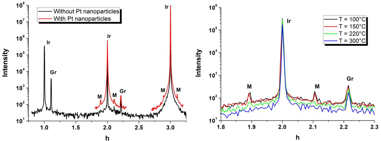
Fig. 2: (Left) Comparison of the GIXRD peak intensities, along the (h00) direction, before and after Pt nanoparticle deposition (sample S3). The moiré peaks are labelled by the letter "M". (Right) Evolution upon annealing of the GIXRD peak intensities, in the (h00) direction, for sample S3.
