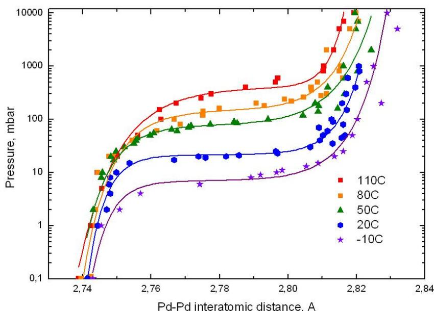
Figure 2. Pressure-composition isotherms obtained from EXAFS analysis.
