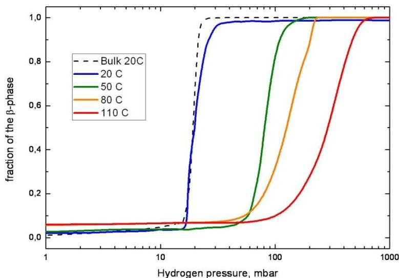
Figure 4. Concentration of PdH  $\beta$ -phase with increasing hydrogen pressure at different temperatures.
