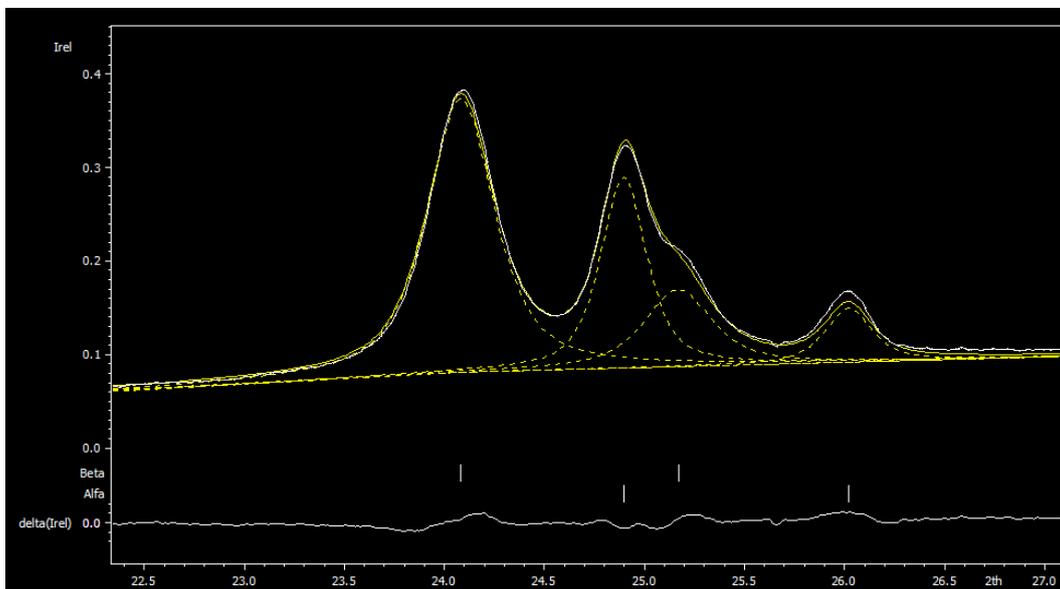
Figure 3. Example of the XRD pattern fitted with two Pd phases.
