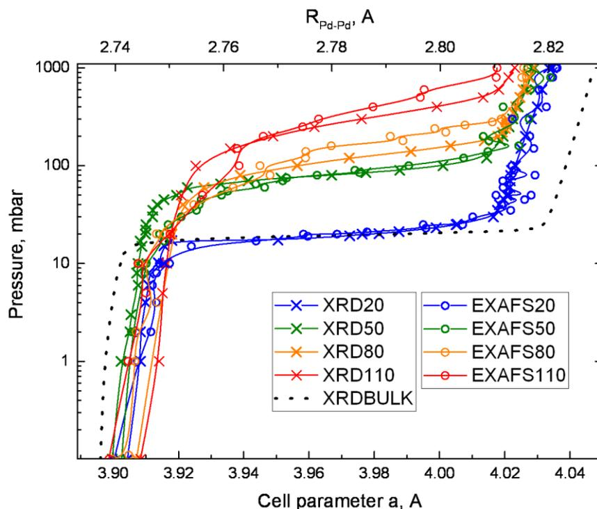
Figure 5. Comparison of the isotherms obtained from XAS and XRD. Black dashed curve correspond to Pd black sample.
