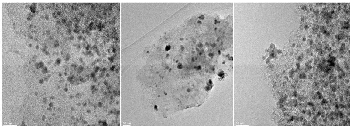
Fig.1. TEM images of Pd/C nanoparticles.
