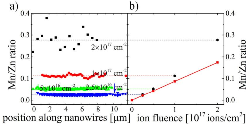
*Figure 2: a) Mn-Zn ratio along the nanowire length for sparse nanowire samples irradiated with the indicated ion fluence of  $175 \text{ keV Mn}^+$ . There is no concentration gradient along the nanowire length. In b) the average ratio obtained for the respective ion fluence is shown in black next to the simulation without sputtering in red (from [2]).*
