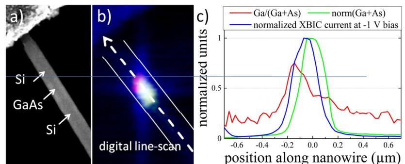
*Figure 1: a) SEM image of a contacted Si-GaAs hetero-nanowire. b) Overlay of the concentration maps of  $\text{Ga}/(\text{Ga}+\text{As})$  and  $(\text{Ga}+\text{As})$  with the XBIC signal and c) plot of these to a normalized scale.*
