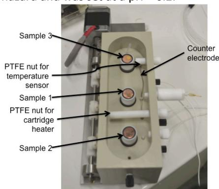
**Figure 1** Cu/Au samples mounted within the peCell prior to filling with simulated uterine solution (SUS). A sensor records the electrolyte temperature closest to the electrolyte outlet port. The cartridge heater heats the electrolyte between Samples 1 and 2, across the width of the cell.
