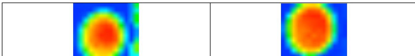
Figure 1. Fluorescence map for two typical porous Si samples electrochemically doped with Er in 12x10 mm scans covering the entire porous area. Blue is the minimum Er content and red is the maximum.
