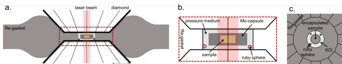
**Figure 2.** (a) A schematic cross section showing the experimental setup with an encapsulated sample loaded together with a few ruby spheres for pressure estimation and surrounded by KCl pressure medium inside the pre-indented Re-gasket. (b) Magnified view of the experimental configuration of the loaded encapsulated sample and laser heating area (red shaded) (c) Axial view of an encapsulated sample.
