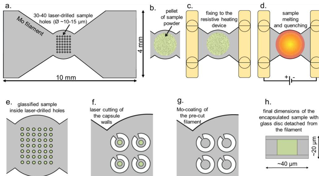
**Figure 1.** A schematic detailing the fabrication technique for the metal encapsulated glass disc samples using the so called ‘filament method’. See main text for more detail explanation.
