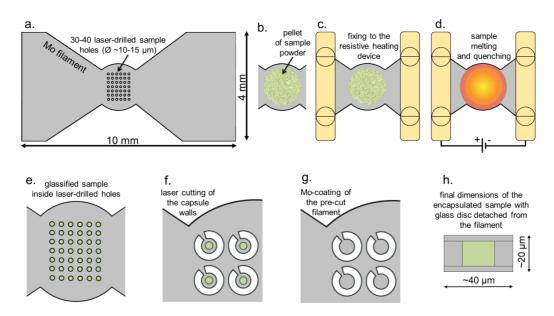
**Figure 1.** A schematic detailing the fabrication technique for the metal encapsulated glass disc samples using the so called 'filament method'. See main text for more detail explanation.
