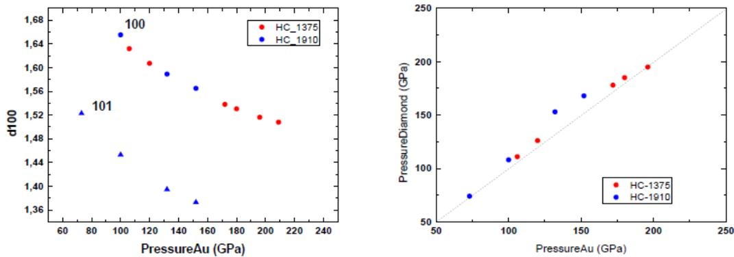
**Figure 1 : Left: Evolution of  $d_{100}$  and  $d_{101}$  of solid  $H_2$  at 300 K in phase. The data of runs HC-1375 and HC-1910 are represented in red and blue respectively. Right: pressure estimated from the diamond anvil phonon versus the one obtained from the volume of a ball of gold embedded in hydrogen.**
