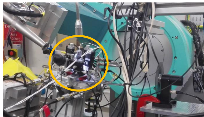
Figure 1. X-AFM mounted on the hexapod at ID03
