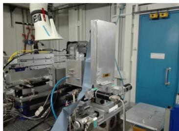
Figure 1 – Left: the AFE readout daughterboard, connected to the sensor testboard, as mounted in the support frame. right: The complete support frame mounted on the ID 17 beamline.
