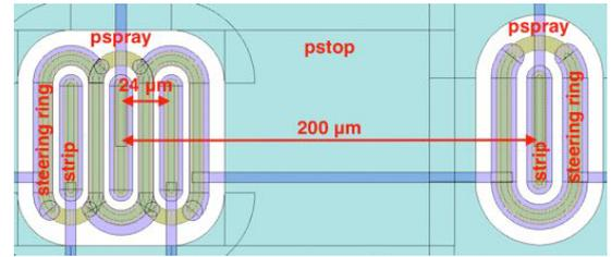
Figure 2: variable pitch sensor geometry
