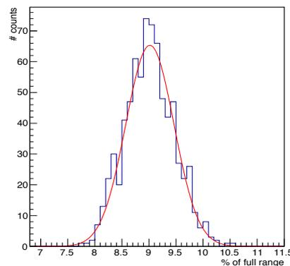
Fig 3: Left: microbeam profile as observed with the 50  $\mu\text{m}$  pitch sensor. Red squares show the centre of mass and average charge for each triplet. Right: amplitude distribution during one single exposure for one single channel.
