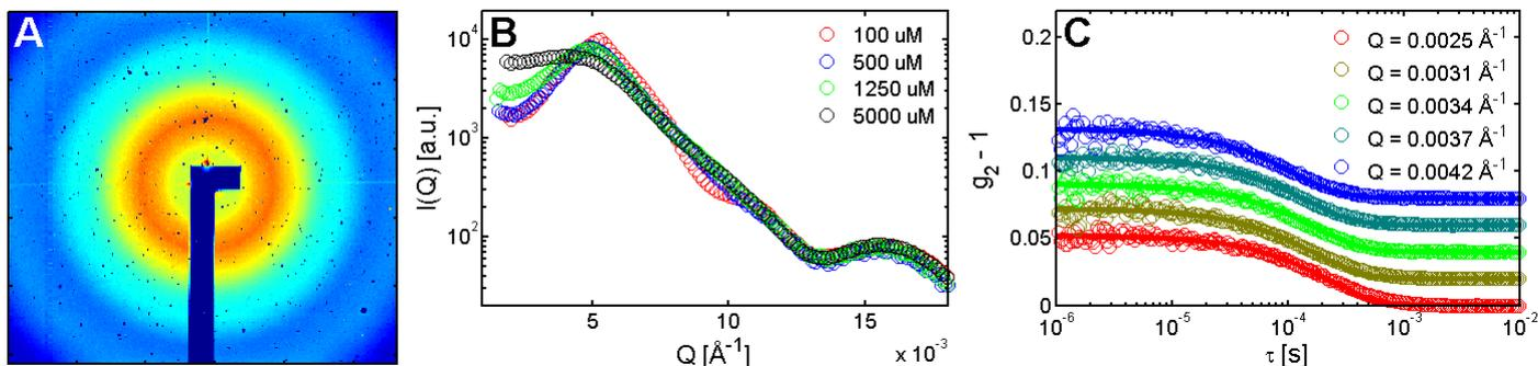
Fig.1 A: Example scattering pattern recorded with the Maxipix 3x1 for a bimodal sample at an electrolyte concentration of 100  $\mu\text{M}$ . B: Azimuthal integrated scattering intensities of a set of 4 samples with different salt concentrations and otherwise unchanged sample parameters. C: Autocorrelation functions of a bimodal sample. The symbols display the measured  $g_2$ -functions, the solid lines are fits. The autocorrelation functions have been offset vertically for better visibility.
