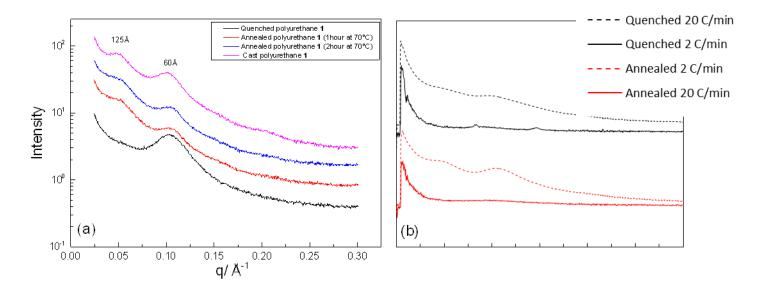
**Figure 1.** Small angle X-ray scattering (SAXS) of polyurethane **1** with; a) different processing histories, b) different cooling rates with respect to different processing histories.
