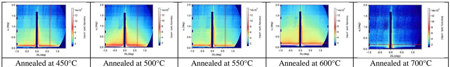
Fig 3. Experimental scattering pictures at room temperature of a porous SiOCH film after an in-situ annealing.
