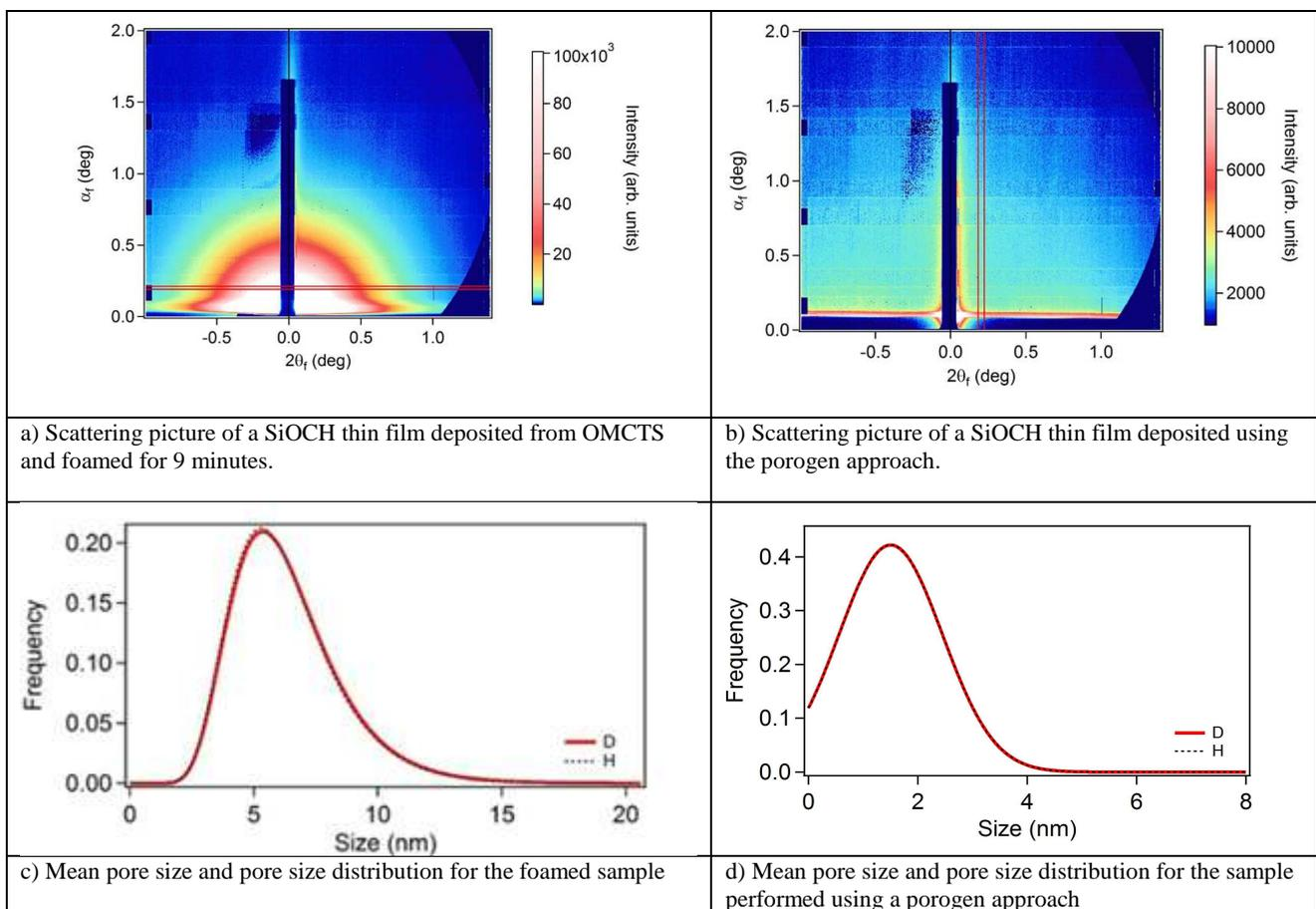
Fig 1. Experimental scattering pictures of porous SiOCH films and pore size distribution deduced from simulation.
