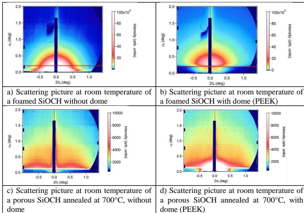
Fig 2. Experimental scattering pictures at room temperature of porous SiOCH films with or without the dome.
