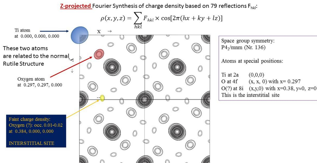
The charge density  $[\rho(x,y,z)]$  map of the projected structure shows four unit cells in which the strong peaks are related to the V atom at (000) and  $(\frac{1}{2} \frac{1}{2} \frac{1}{2})$  as well as to the oxygen atom at (0.297, 0.297, 0.000) and the symmetrically equivalent ones.
