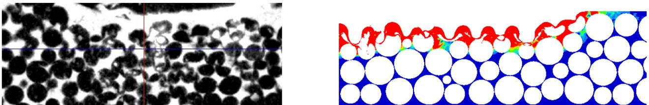
**Fig. 2.** X-ray micro-tomography of a polyurethane foam recovered after a laser shock applied onto the upper surface, showing pore collapse after buckling and rupture of the polymer matrix (left), and simulation of the foam response to laser shock loading, showing the early stage of wave propagation 0.25  $\mu\text{s}$  after the shot (right).
