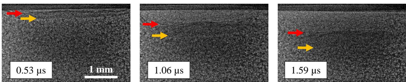
**Fig. 1.** X-ray phase contrast snapshots of a polyurethane foam at successive times after a laser shock applied on the upper surface, showing the propagation of a compaction wave (red arrows, 0.39 km/s mean velocity), preceded by an elastic precursor (yellow arrows, 0.76 km/s mean velocity) which can be evidenced more clearly by dividing by the static, pre-shock image (see ref. 3 for details).
