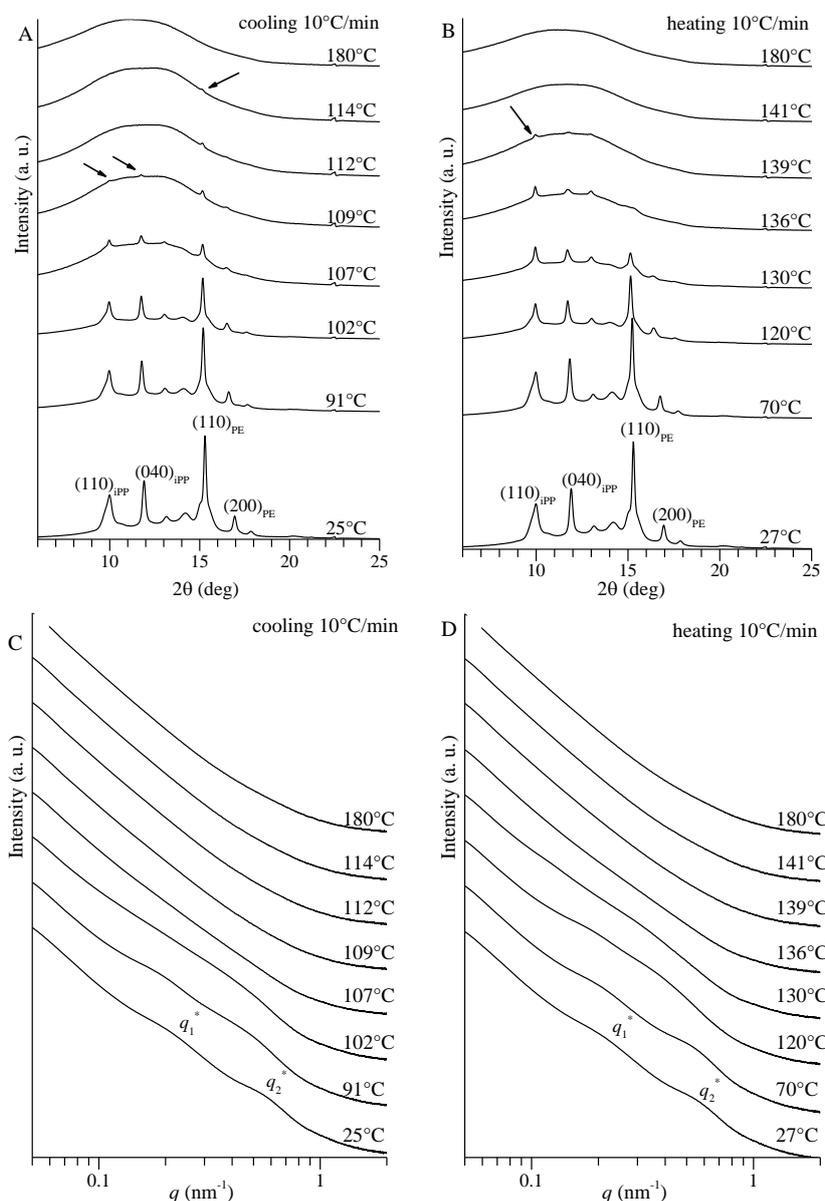
**Figure 1** WAXS (A,B) and SAXS (C,D) profiles of the sample RDG-1-91 ( $f_w \text{ iPP} = 0.74$ ) belonging to the series of iPP-*b*-PE BCPs, recorded during cooling and heating scans at 10°C/min at the indicated temperatures.
