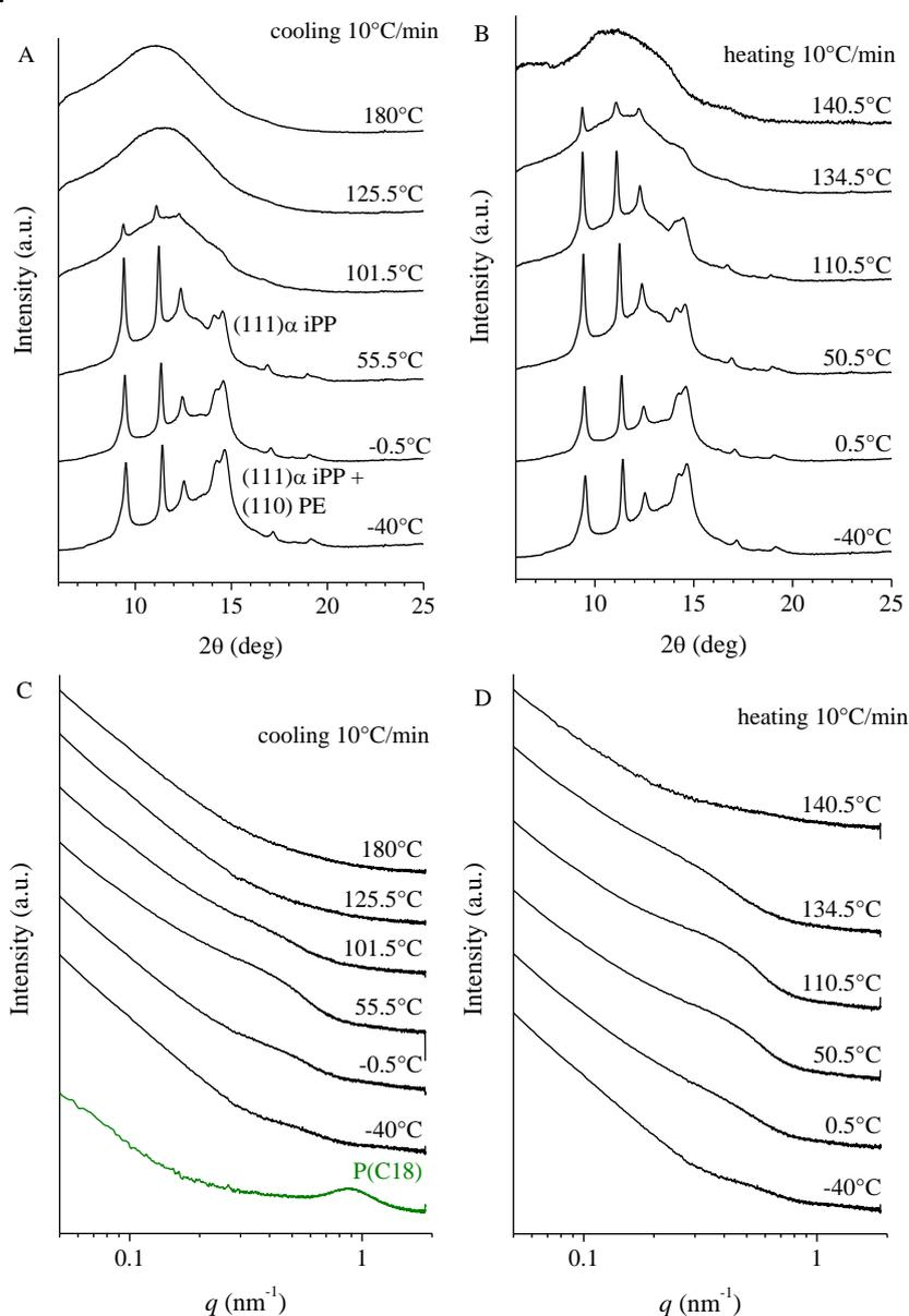
**Figure 2** WAXS (A,B) and SAXS (C,D) profiles of the sample RDG-1-148 ( $f_w \text{iPP}=0.49$ ) belonging to the series of iPP-*b*-(P-*co*-C18), recorded during cooling and heating scans at  $10^{\circ}\text{C}/\text{min}$  at the indicated temperatures.
