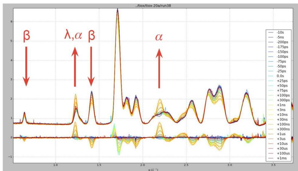
**Fig. 2** Azimuthally integrated differential powder scattering signal for different time delays. Uppers series of curves are the absolute intensities, lower series of curves is the resulting differential signal.
