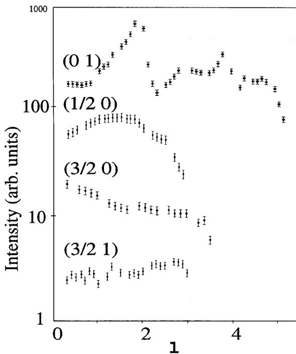
Figure 1: Selected rod profiles measured from  $\text{TiO}_2(110)1 \times 2$ .
