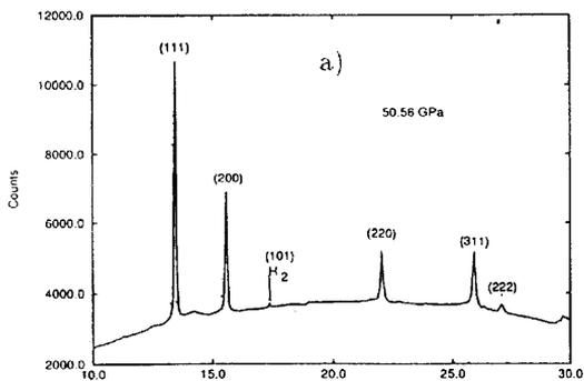
Figure 1: a) Diffraction patterns of NiH from the 1st run. No structure changes were found. The (101) peak of a powder diffraction pattern from molecular hydrogen is also observed. b) Diffraction pattern at 123 GPa
