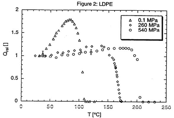
In figure 2, the new result of LDPE at 540 MPa is given together with the former studied behaviour at lower pressures [2]. It can be seen, that the slope of the invariant-pressure curves decrease with increasing pressure. This can be explained by the approach of the thermal expansions of the purely crystalline and the purely amorphous phases in the sample.
