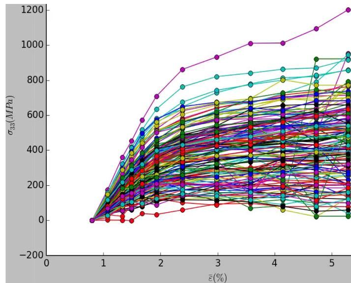
Figure 2. Stress state of individual R117-680 grains, following the loading direction, as function of the macroscopic strain.
