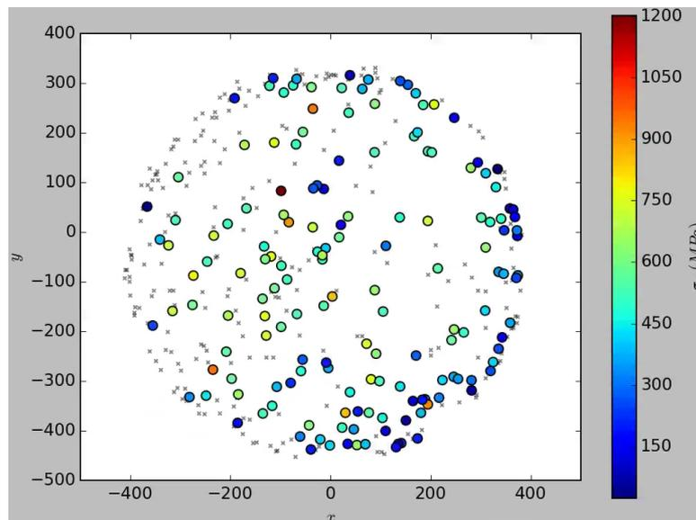
Figure 3. Radial positions and stress state of individual grains in the sample "R117-680".
