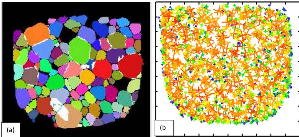
**Figure 1. Unstrained AH35 sample containing more than 1400 grains in the probed volume: (a) DCT reconstruction, (b) 3DXRD result.**
