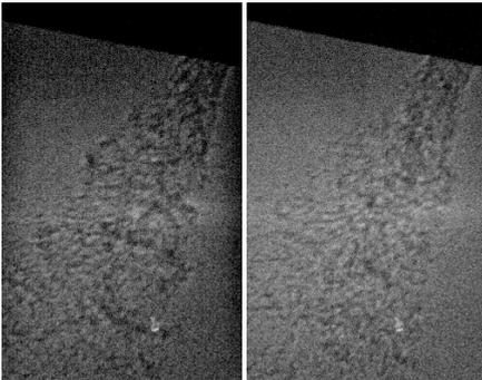
Figure 3: Comparison of two different propagation distances: 5.3 m (left) and 4.5 m (right) (150 bar injection pressure)
