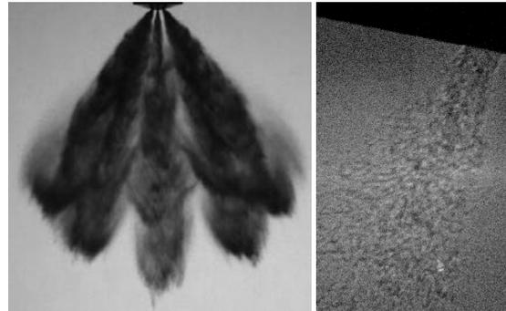
Figure 4: Shadowgraphy image of the whole spray (left) and x-ray image of the near nozzle region (right) (150 bar injection pressure)
