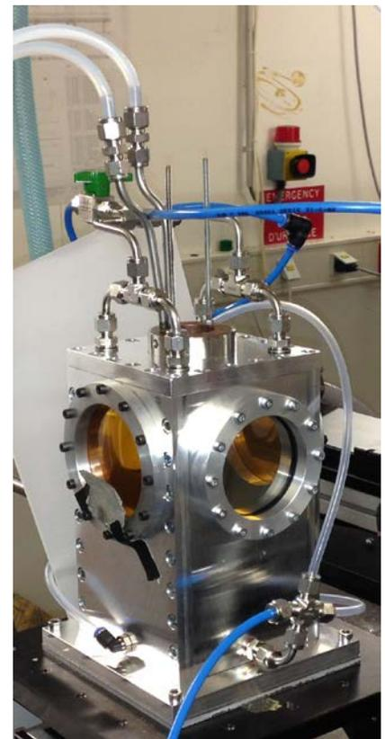
*Figure 1: Constant volume chamber used for the spray measurements*
