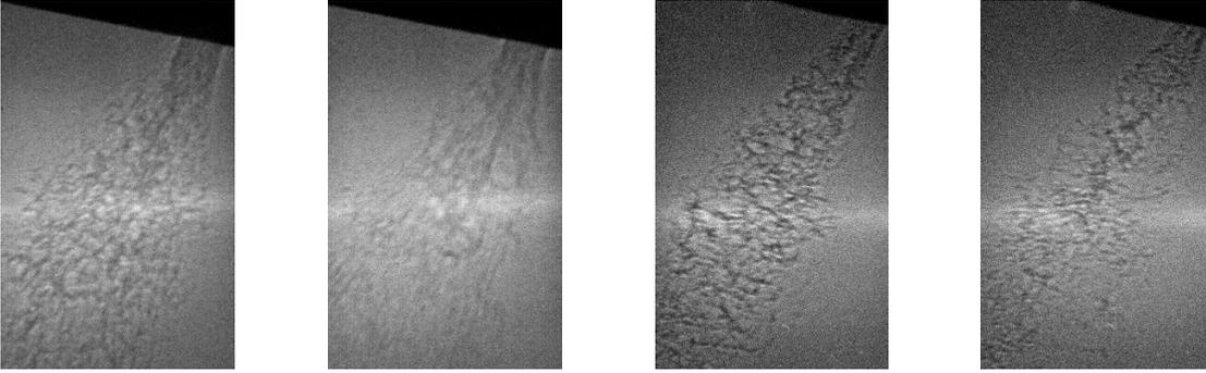
Figure 2: Comparison of the different scintillator materials at two different injection pressures (from left to right): LuAG:Ce, 50 bar; LuAG:Ce, 250 bar; LYSO:Ce, 50 bar, LYSO:Ce, 250 bar
