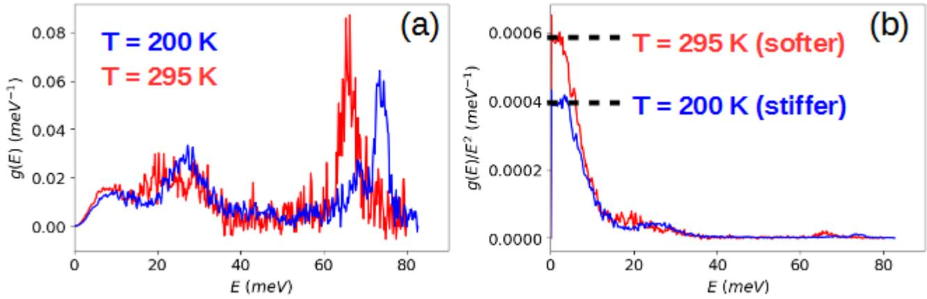
Figure 1. (a) Fe-DOS at two different temperatures of **C224**. (b) Reduce density of states at two different temperatures of **C224**.
