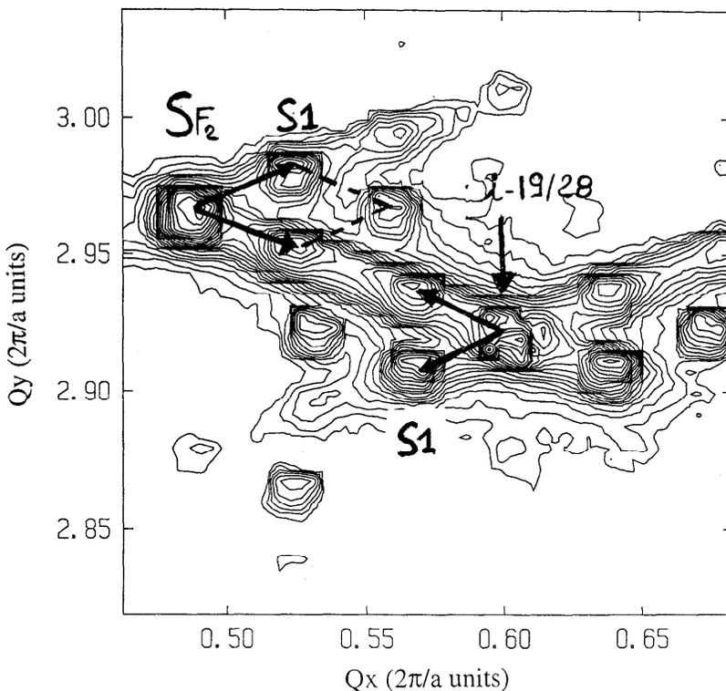
Figure: 2D isointensity map around the 19/28 main i- Bragg reflection . A large number of S 1 satellite reflection observed around he i- and SF2 type reflection.
