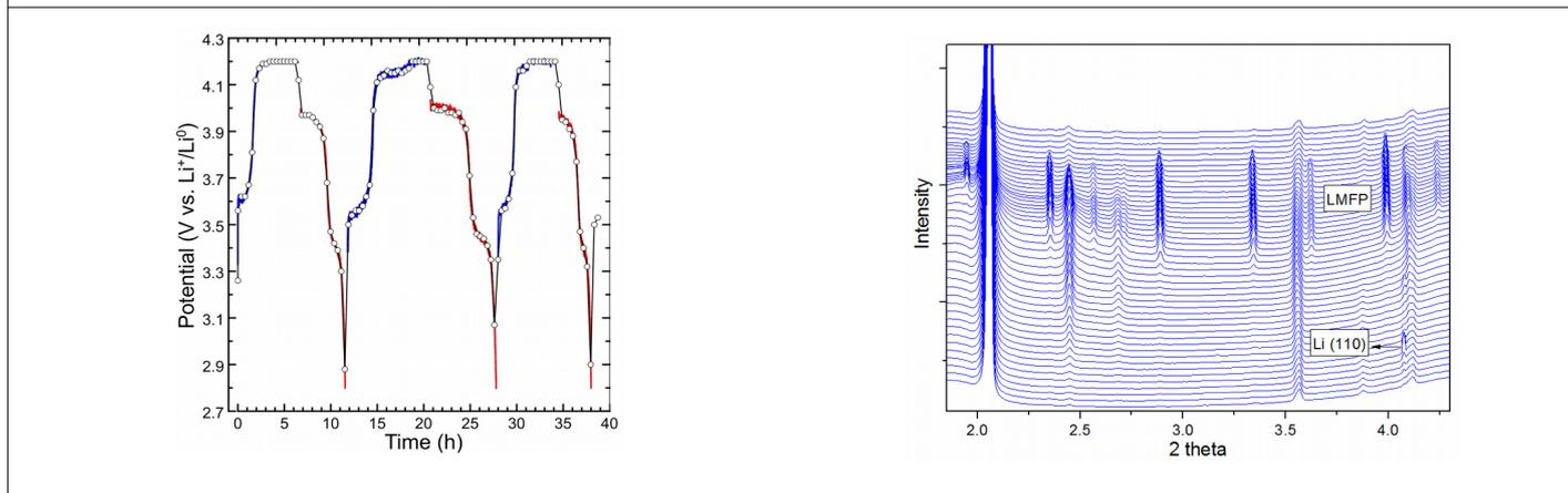
**Figure 3.** Potential vs. capacity of a Li/LMFP battery with a single-ion conductor SPE. (blue) charge step, (red) discharge step, and the open symbols are the X-ray illumination.
