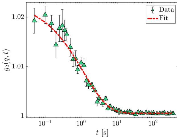
Fig.1: Example of correlation function obtained for the  $\text{B}_2\text{O}_3$  glass on the peak of the structure factor,  $q \sim 15 \text{ nm}^{-1}$ , at the temperature  $310^\circ\text{C}$ . The exposure time for this particular measurement was set to 50ms and the total number of images is  $1.8 \cdot 10^5$ . Figure from ref. [4].
