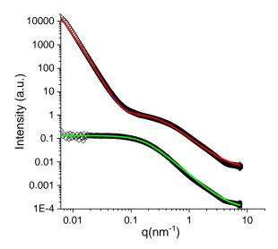
Maltodextrin-based systems. Not cross-linked (bottom) and cross-linked (top). Fitting lines have been obtained with a polydisperse polymer coil model (green line) or with the same model + Porod's regime at low q values.
