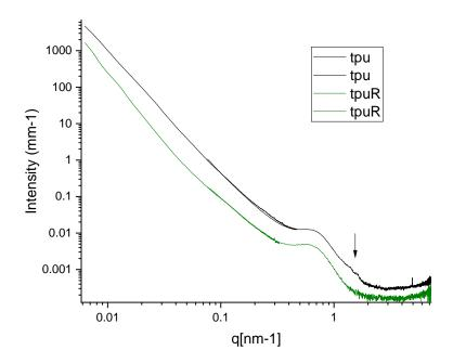
Aligned samples display peaks in the q region  $1 < q < 2 \text{ nm}^{-1}$  that disappear in the random- prepared samples. The small peak at  $q = 1.4 \text{ nm}^{-1}$  is characteristic for thermoplastic polyurethane as visible in the scaffolds prepared by lyophilisation from mold at 8% or 10% concentration)
