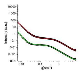
Dextran-based systems. Not cross-linked (bottom) and cross-linked (top). Fitting lines have been obtained with a polydisperse polymer coil model  $+\ q^{-s}$  regime at low q values ( s=3.2 green, s=2.7 red)
