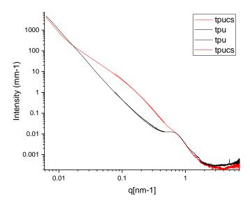
TPU are linear block copolymers consisting of thermodynamically incompatible soft (SB) and hard (HB) blocks that undergo a microphase separation. The broad peak at  $q = 0.7 \text{ nm}^{-1}$  is related to a characteristic distance depending on the length of soft and hard blocks.
