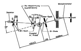
Fig.1. Experimental set-up for the high energy powder diffraction experiment
