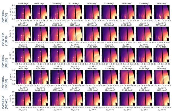
The Figure above shows the heating cycles of C10-DNTT on top of different sub-layers. The sublayers consist of PVPh cross-linked with HDA to different degrees. All films show the phase transition
