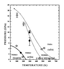
p-T phase diagram of KNbO<sub>3</sub>.
