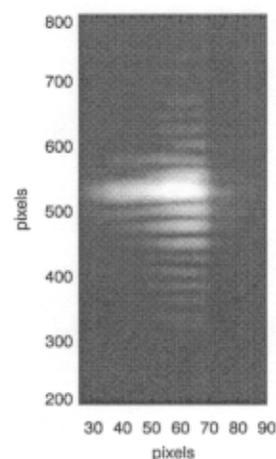
Figure 2. CCD image of modes exiting an empty waveguide for a gap width of 600 nm.
