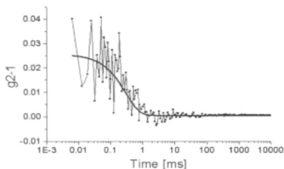
Figure 3 Time correlation function for Ø 120 nm SiO<sub>2</sub> spheres inside a 2 micrometer wide waveguide. The solid line is the theoretical decay for single particle diffusion in bulk.
