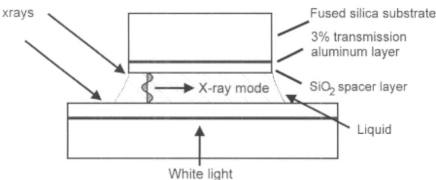
Figure 1 Schematic drawing of the x-ray waveguide setup
