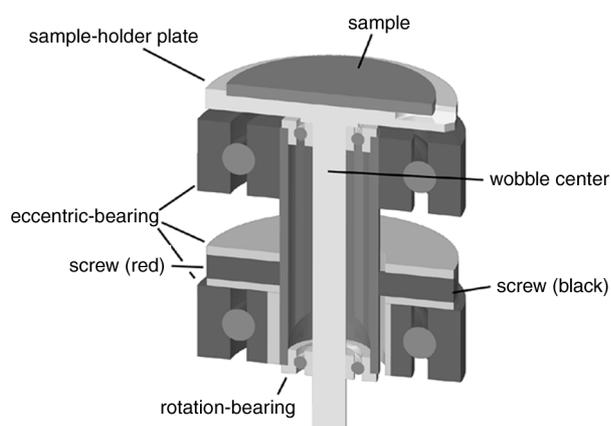
Figure 1. A schematic diagram of the sample wobbling mechanism tested in the first part of the experiment.
