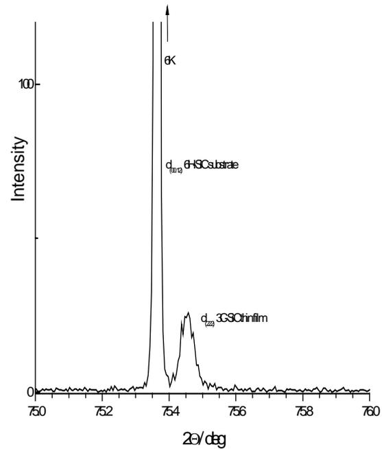
Fig. 2: X-ray diffractogram of the 3C-SiC thin film ( $\approx 1\mu\text{m}$ ) on 4H-SiC wafer demonstrates the intensity ratio
