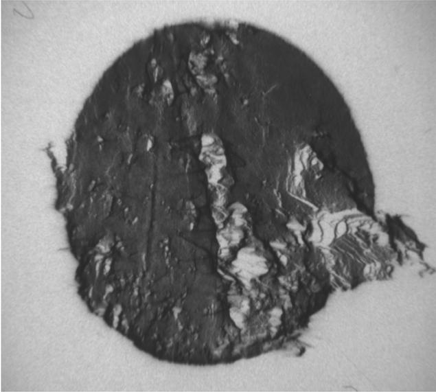
Fig. 1: Asymmetric 10.9-reflection topograph of the 4H-SiC wafer. The sample oscillating has compensated the wafer bending.
