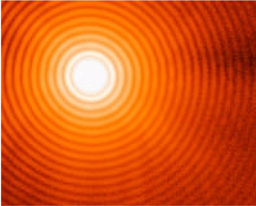
Fig. 1. Airy diffraction pattern of a coherently illuminated 10 micron pinhole at  $\lambda=1$  nm. On this logarithmic intensity plot, 24 rings can be observed.
