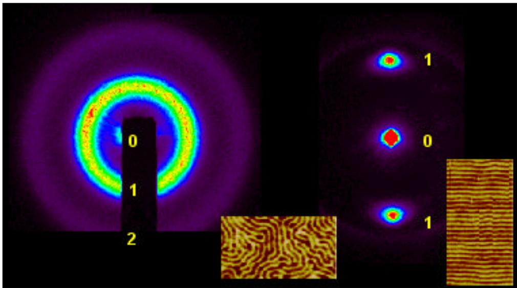
Fig. 3. Diffraction patterns taken taken in transmission at the Gd  $M_5$  edge of GdFe stripe domains ( $T=20$  K). Left: disordered stripes give rise to a “magnetic powder” ring. Right: Magnetically aligned stripes act as a grating and produce a series of maxima.
