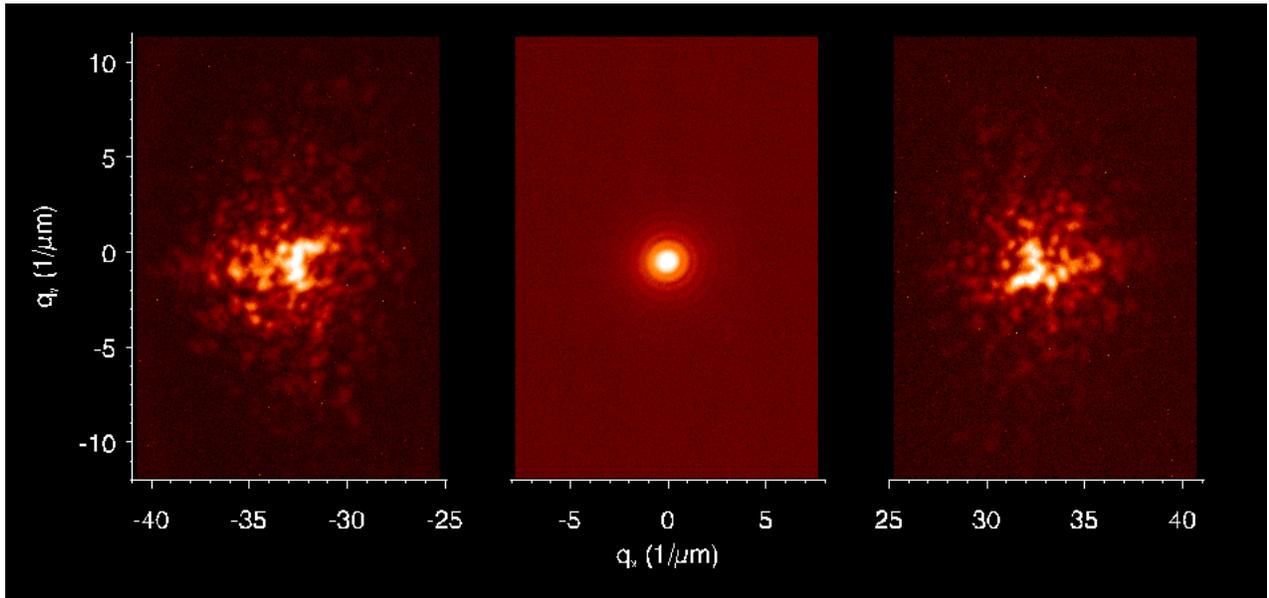
Fig. 5. 1<sup>st</sup> order speckle intensity of aligned stripes around the transmitted 10  $\mu\text{m}$  primary beam. The latter shows clear Airy fringes, demonstrating the coherence of the light. The speckle images are centralsymmetric and are correlated for 94%.
