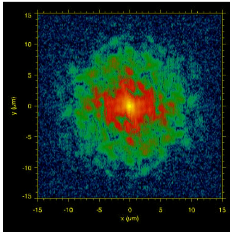
Fig. 6. Magnetic correlation function obtained by Fourier transforming the speckle intensities of Fig. 5.
