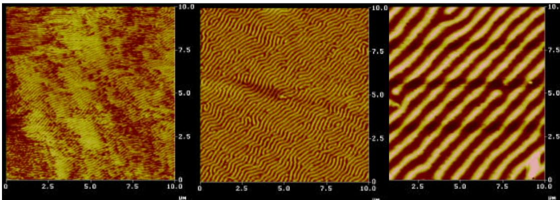
Fig. 2. Magnetic Force Microscopy image of the stripe domains in GdFe films of various thickness, showing the tunability of the stripe period. The same can be achieved by varying the composition.
