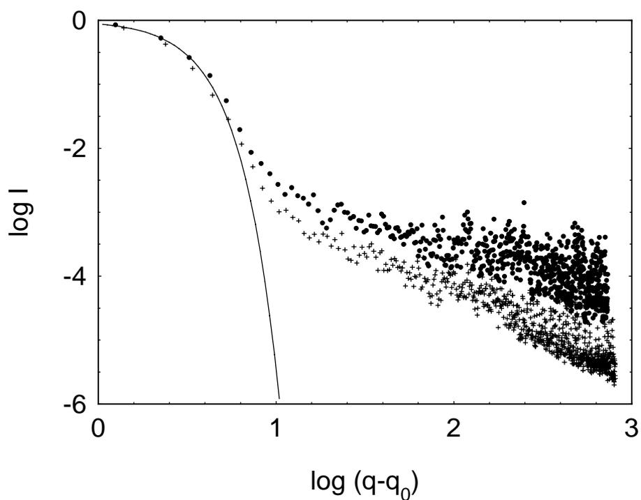
Figure 2. Profile of the first order diffraction peak of the block copolymer showing the Caillé wing at large  $q-q_0$ ; the full line is a fit of a Gaussian resolution function to data in the region of small  $q-q_0$ . Symbols: ● 25°C, + 50°C.
