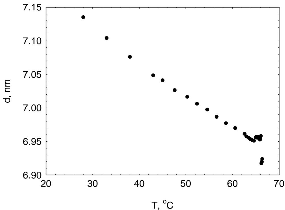
Figure 1. Temperature dependence of the smectic period of the block copolymer melt. Note the small but significant *increase* just before the ODT
