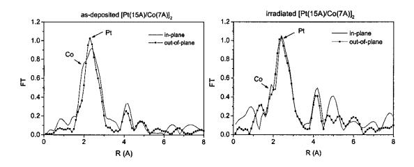
An important anisotropy in the local structure around cobalt is observed for the non-irradiated sample. A larger number of first neighbour Pt atoms is observed in the out-of-plane direction, consistent with the presence of perpendicular magnetic anisotropy. This anisotropy practically disappears from the main FT peak in the irradiated sample and explains the change of easy magnetisation direction from out-of-plane to in plane direction.
