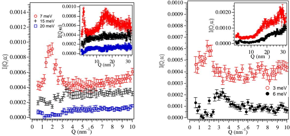
Figure 1. Dynamic structure factor in the Brillouin region at different energies. a)  $\text{Li}_2\text{O}-2\text{B}_2\text{O}_3$  and b) CKN. The inset shows the full experimental Q-range. The spectra have been shifted vertically for clarity.
