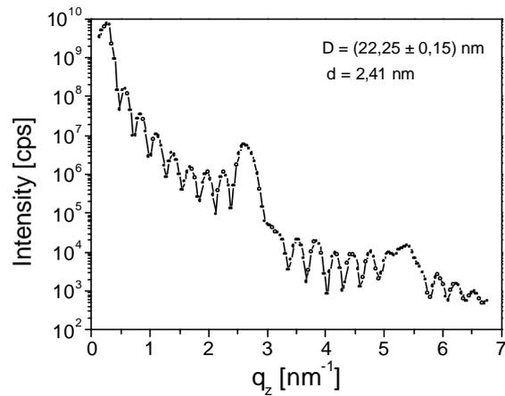
**Fig. 2: Specular reflectivity of a sample with 9 ML of HBC on covered silicon**
