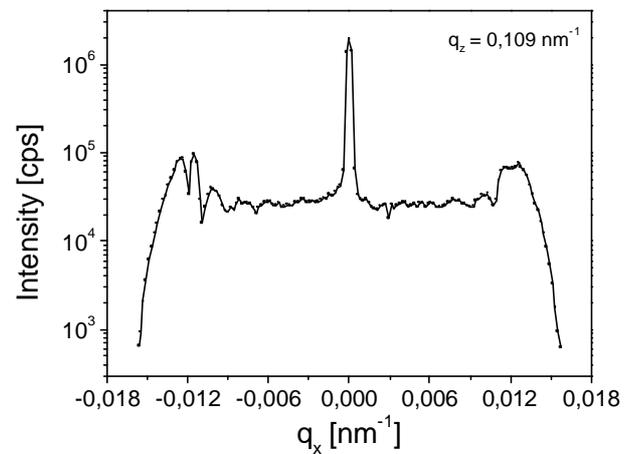
**Fig. 4: selected transversal-scan from fig.3 9 ML of HBC on PEI covered silicon**
