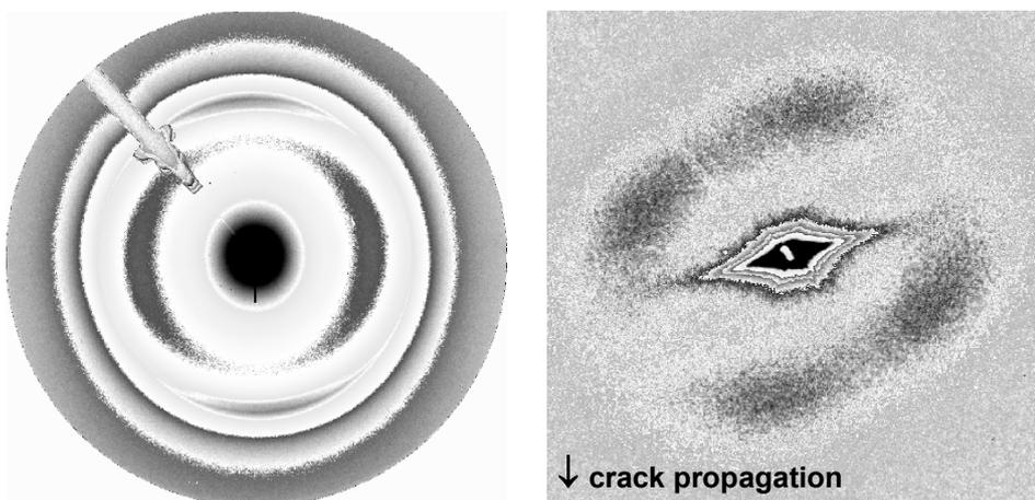
Fig. 2: Representative WAXS and SAXS 2D-patterns of PA6 in the near crack region (zone of strongest deformation: primary macroscopic crack end)
