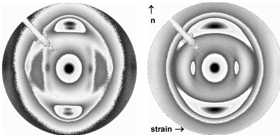
Fig. 1: Representative WAXS 2D-patterns of a stretched dumb-bell of PA6 (left: skin - dominated by  $\alpha$ -modification, right: core - dominated by  $\gamma$ ; n: normal direction of specimen, strain: stress direction)
