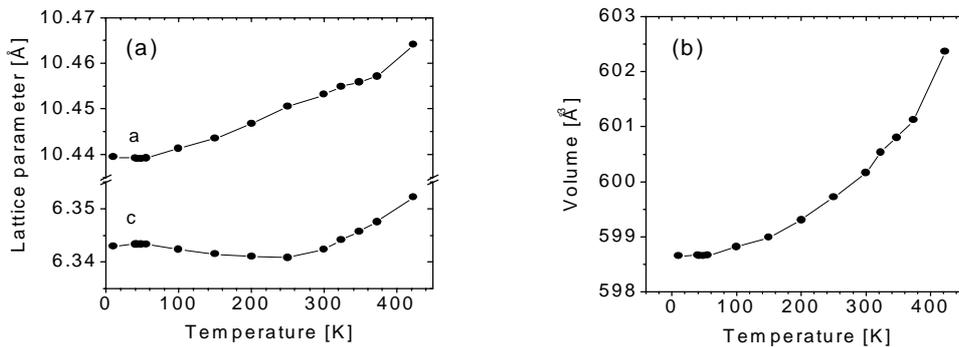
Fig.1 Temperature dependence of the lattice parameters (a) and unit cell volume (b) of  $\text{CaMn}_7\text{O}_{12}$  in the trigonal phase. The lattice parameters are given in the hexagonal setting.
