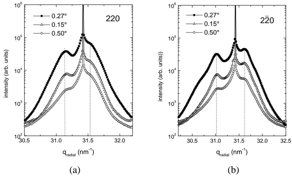
**Fig.1:** Radial scans of triple crystal grazing incidence diffraction (integrated PSD signal) on a 10 period InP/InGaP QD superlattice (a: 220, b:  $\bar{2}20$ ) recorded at different angles of incidence.
