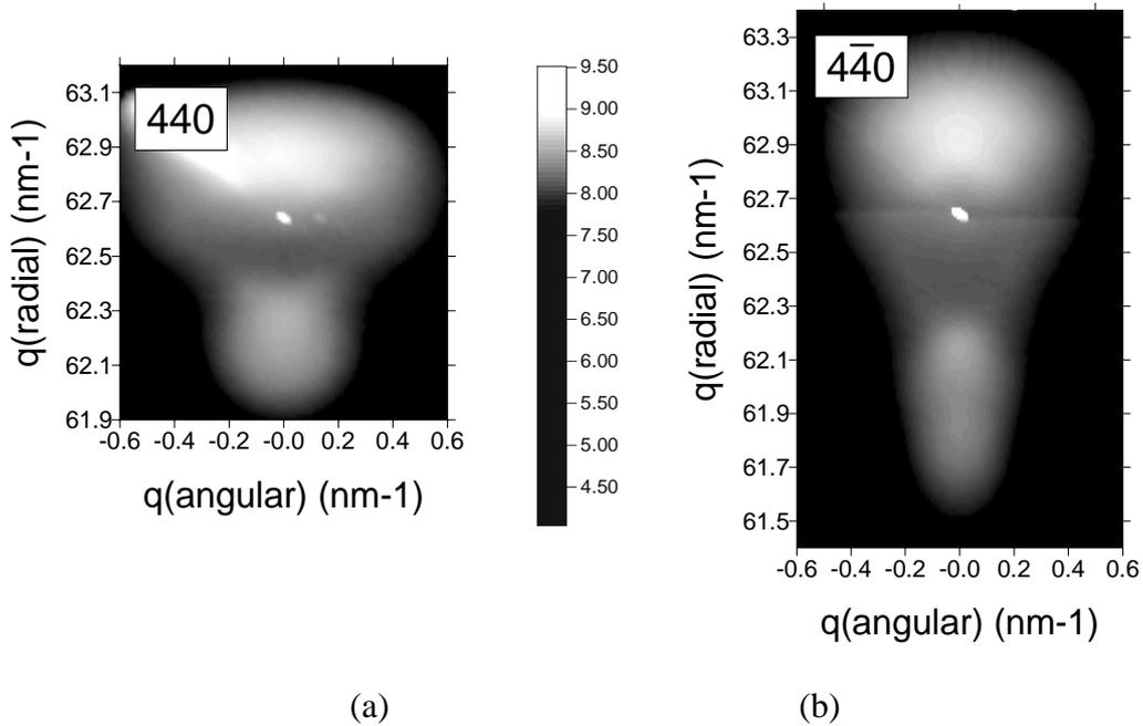
**Fig.2:** 2D cut through reciprocal space (at  $q_z = 0.38 \text{ nm}^{-1}$ ) around the (a) 440 and (b)  $\bar{4}40$  reciprocal lattice points. The intensity scale is varying logarithmically as shown by the grey scale.
