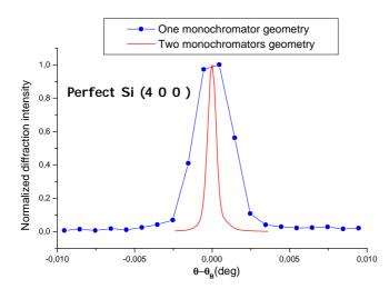
Fig.1 Instrumental function with (red solid line) and without (blue line with dots) a secon monochromator dispoersing in the horizontal plane
