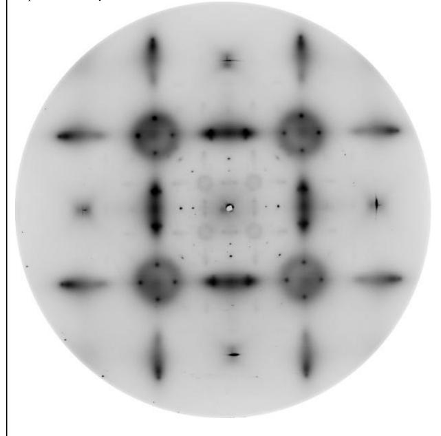
Fig 1. Short and long range order in the  $Pt_4V$  measured on ID15B **References**
