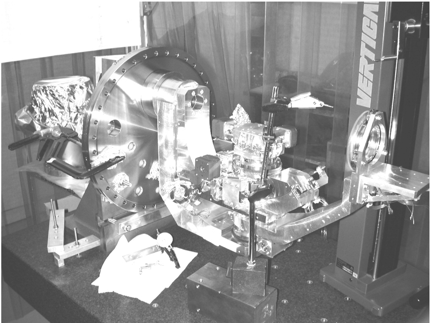
Figure 1 uhv goniometer undergoing first phase tests at the RMP factory.
