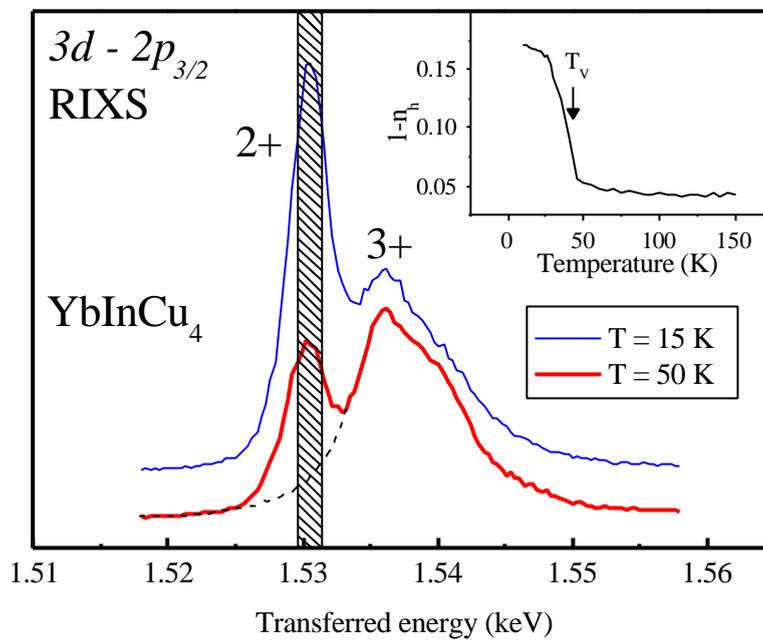
Figure 2. Ytterbium  $L\alpha_1$  RIXS spectra in  $\text{YbInCu}_4$  excited at the maximum of the  $\text{Yb}^{2+}$  resonance of Figure 1 ( $h\nu_{\text{in}} = 8945 \text{ eV}$ ). The small change of valence ( $\Delta n_h = 0.13$ ) results in a large change of the divalent peak intensity. The inset shows the continuous intensity evolution of the number of  $f$ holes, measured by monitoring the shaded area indicated on the RIXS spectra.
