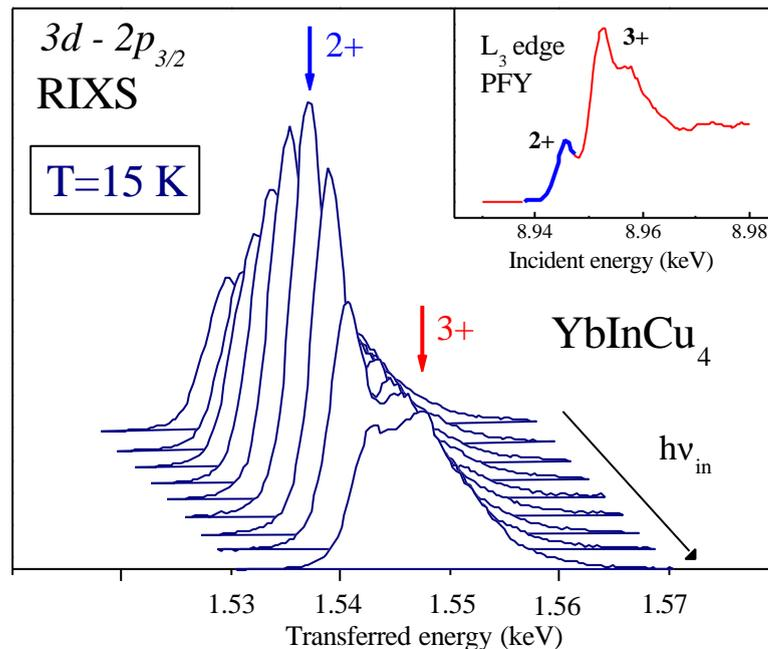
Figure 1. RIXS spectra of ytterbium in  $\text{YbInCu}_4$  below the transition temperature ( $T_V = 42$  K). The incident energy was scanned in the region of the  $\text{Yb}^{2+}$  signal (thick part of the Partial Fluorescence Yield absorption curve in the inset). At its resonance the divalent peak dominates the spectrum.
