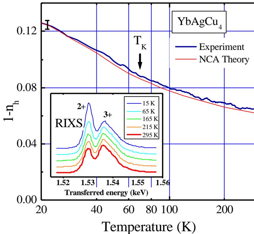
Figure 3. Temperature dependence of the  $\text{Yb}^{2+}$  RIXS signal of  $\text{YbAgCu}_4$ , measured as in Fig.2. The experimental signal has been normalized to the incident photon intensity, and a constant term from the tail of the  $\text{Yb}^{3+}$  signal has been subtracted. The measured intensity has been converted into  $(1-n_h)$  values by adopting the XAS value  $n_h(15 \text{ K})=0.87$ . Raw RIXS spectra at representative temperatures are shown in the inset.
