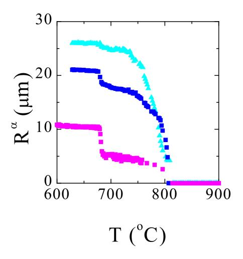
**Fig. 1**: The radius  $R^{\alpha}$  of three individual ferrite grains as a function of temperature during the phase transformations in a 0.22 wt.% C steel. The sample was cooled at a rate of 5 °C/s.
