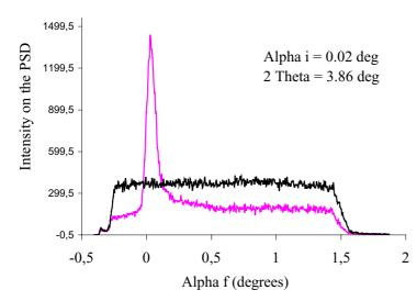
Fig. 3 Intensity of Bragg reflection as a function of  $\alpha_f$  at the (200) peak of the film (pink) and bulk sample (black), respectively. Only the film sample shows the expected maximum at the critical angle  $\alpha_c = 0.02^\circ$ .
