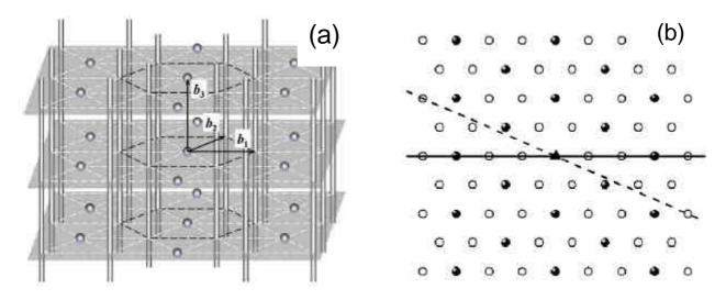
Figure 1. (a) Sketch of the reciprocal lattice of randomly stacked hexagonal close packed crystals. (b) Top view of the reciprocal lattice illustrating the orientation of the Ewald sphere in Fig. 2 (solid line) and Fig. 3 (dashed). The closed symbols correspond to lines of localised reflections (spots) while open symbols display the position of rods. The triangle marks the line of spots going through the origin of the reciprocal space.
