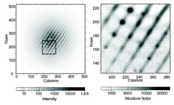
Figure 2. (left) Raw diffraction pattern I(q) measured for the crystal orientation illustrated by the solid line in Fig.1b. The straight beam is absorbed by a small beam stop in the middle of the detector. (right) Magnified view of the structure factor S(q) profile within the area marked on the left panel.
