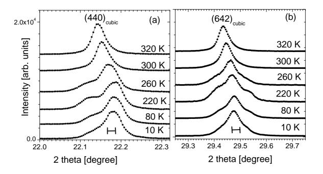
Fig. 1 Representative parts of the SR powder diffraction patterns of  $CaCu_{0.3}Mn_{6.7}O_{12}$  around the (440) and (642) cubic Bragg peak positions are shown in (a) and (b), respectively. Solid circles represent measured data and the lines are shown to guide the eye. The patterns measured at different temperatures are shifted vertically for clarity. The short horizontal line indicates the instrumental FWHM estimated with a Si-NIST standard.
